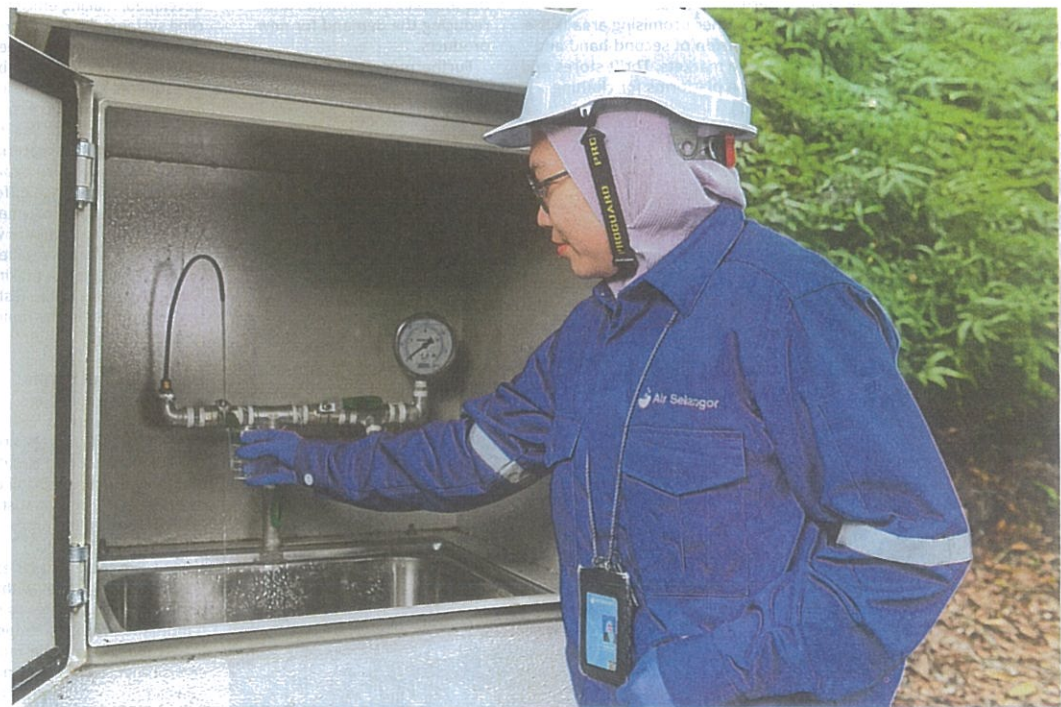
Air Selangor conducts regular water sampling and analysis at its treatment plants, with samples tested every two hours by a team of chemists and microbiologists to identify and address any impurities or contaminants before the water is distributed to the public.
