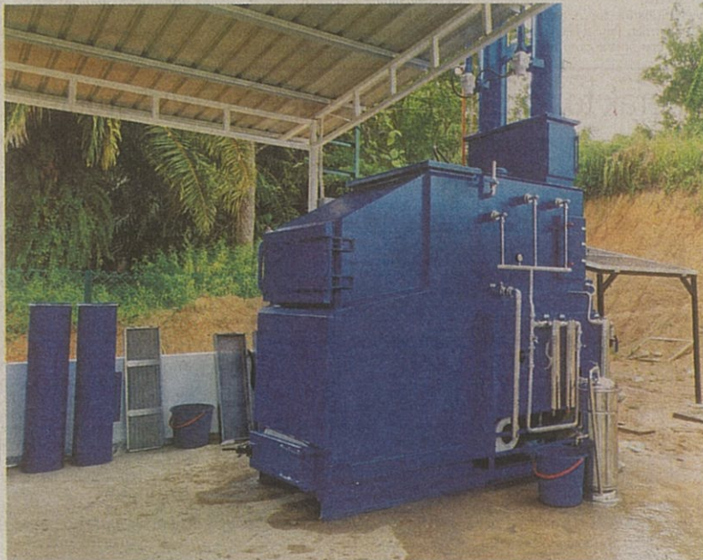
The waste elimination machine is designed to be compact, at only two metres wide and five metres long, and can convert 500 to 900 litres of mixed solid waste to ash every hour.
