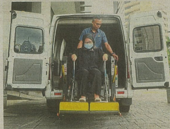
Shazali (standing) demonstrating how the tail lift in one of MBSA's modified vans is used to move a wheelchair user into the vehicle.
