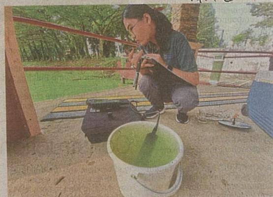
A researcher measuring dissolved oxygen levels with a multiparameter device.
